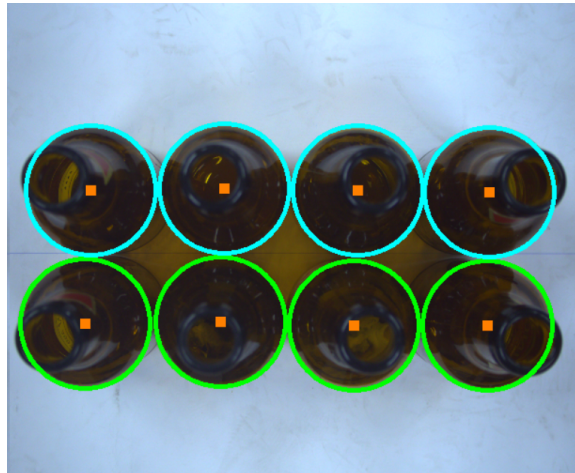
Figure 3.2: Circle detection using the cv.HoughCircles function
