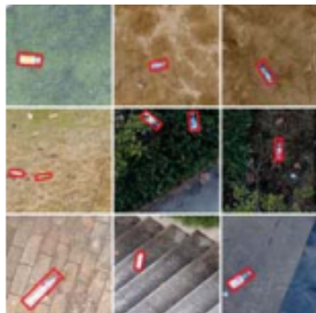
Figure 1.7: UAV images with detection using oriented bounding boxes (Wang et al., 2018)
