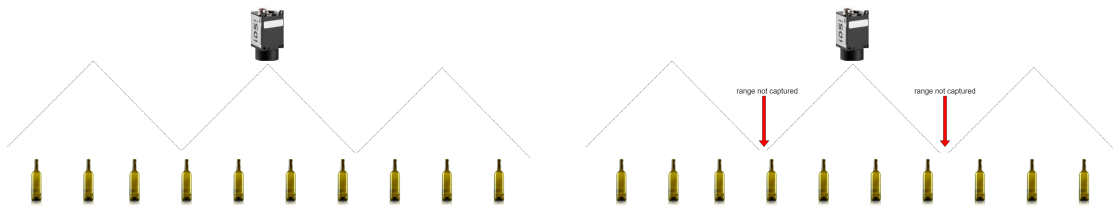
Figure 4.3: Frame capture without overlap at ideal points (left). Frame capture without overlap within intervals, but not exactly at the ideal points (right).
