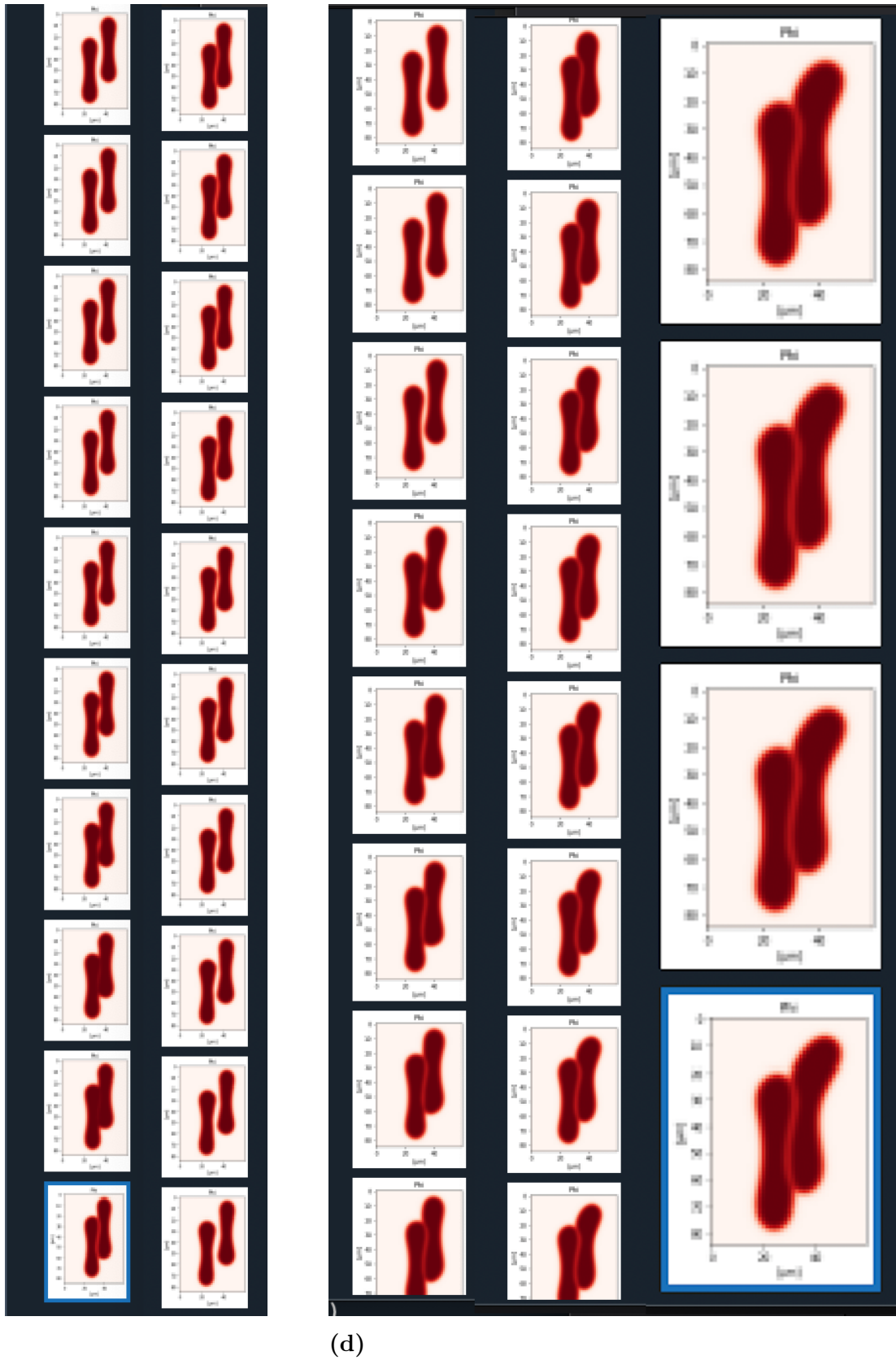
Figure 5.3: Sequence of images (top to bottom, left to right) of the simulation for different values of fluid viscosity: a) 10 ; b) 10^{-2} ; c) 10^{-7} ; d) 10^{-20}
