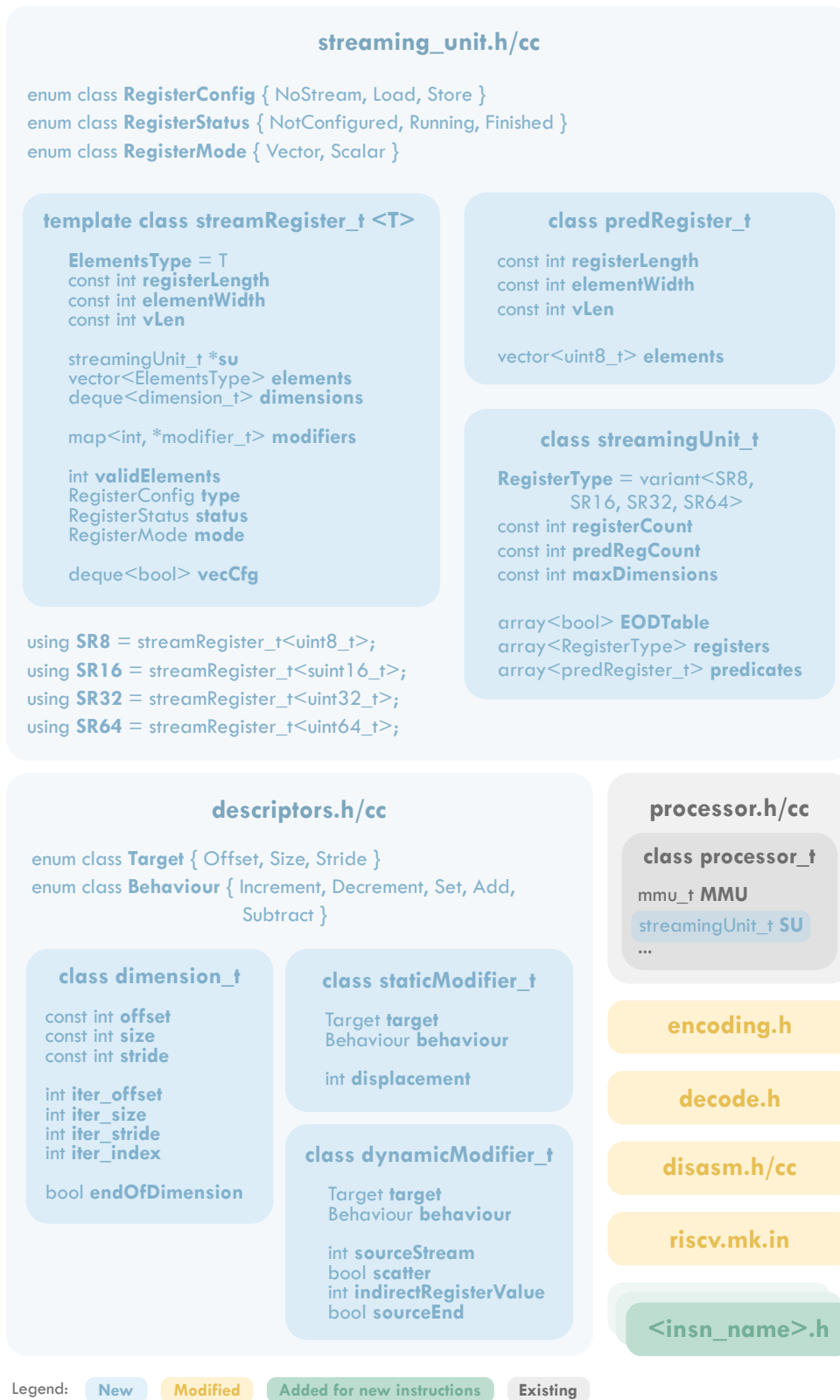
Figure 3.2: Diagram of added and modified structures and files on Spike .
