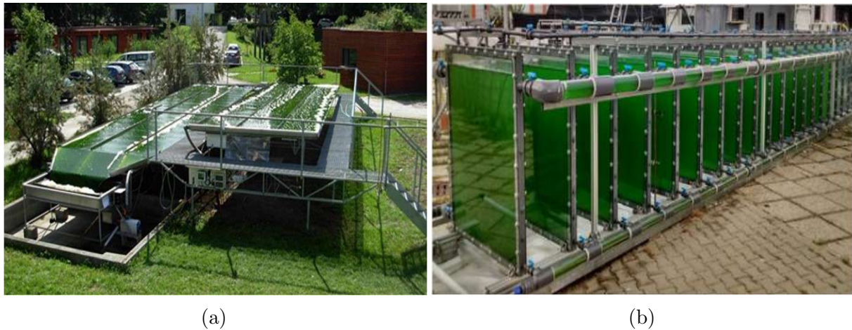
Figure 2.2: (a) Open photobioreactor - thin layer system, from [19], and (b) close photobioreactor - flat-plate system, from [20].
