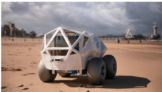
Figure 5 - BeachBot developed by Project.BB roaming a beach searching for cigarette butts to catch with its frontal tool located below the dome. [10]
