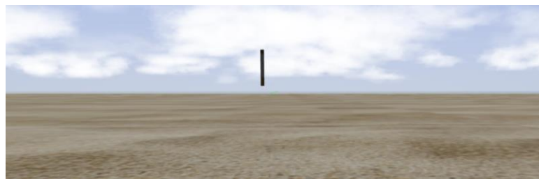
Figure 23 - Litter affected by the buoyancy plugin on Gazebo with vertical orientation instead of horizontal.
