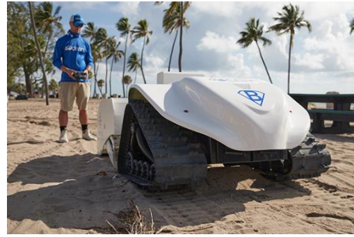
Figure 4 - BeBot, developed by The Searial Cleaners, controlled by an operator performing beach cleaning. [9]
