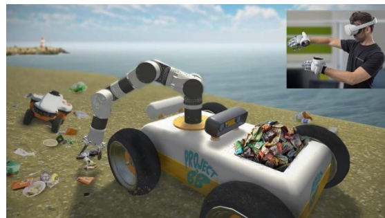
Figure 6 - New concept robot to catch litter having a virtual operator controlling a robotic arm through a VR kit. [10]
