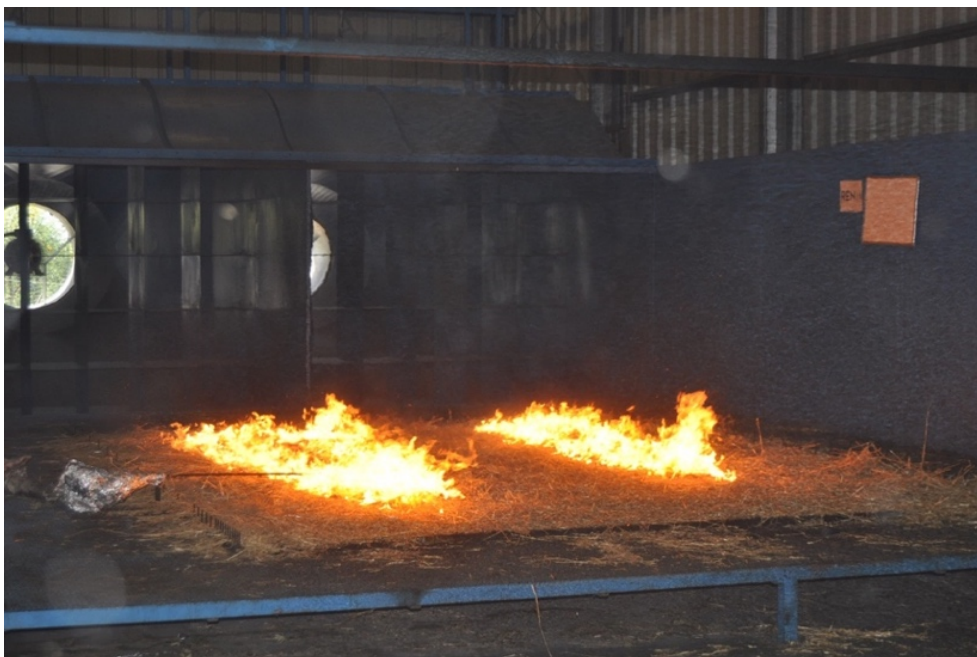
Figure 17: a) Geometry of two parallel fire lines in symmetrical conditions. b) General view of the combustion tunnel of the Forest Fire Research Laboratory of the University of Coimbra. The length of the working section is 8m and the width is 6m. The maximum flow velocity is 8\text{m}\cdot\text{s}^{-1} . The position of the infrared camera and of the visible camera can be seen on the top left of the image, placed in the lifting platform. c) View of the Combustion Tunnel (CT) of the Forest Fire Research Laboratory of the University of Coimbra during the test 2-D2U2.
