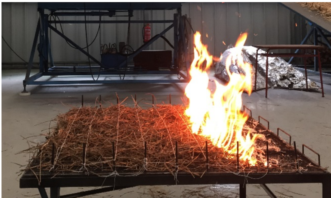
Figure 18: Determination of the basic Rate of Spread R_o in a combustion table with 1 \times 1 \text{m}^2 with a fuel bed of pine needles. The white cotton lines are separated by 10cm of distance and are used to determine the ROS at each distance. The fuel bed load is the same that was used in the experimental tests. This analysis was made for each experimental test.
