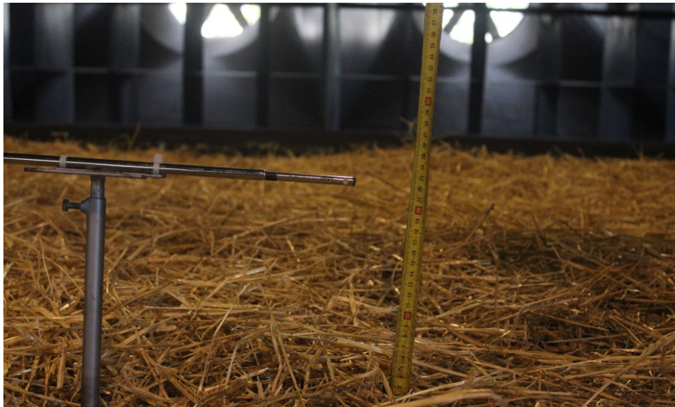
Figure A1: a) Distribution points P_{x,y,z} where wind velocity was measured for wind velocities 1, 3 and 5\text{m}\cdot\text{s}^{-1} in the OX axis. b) KimoAMI 300 hot-wire probe (Kimo Instruments, Montpon-Ménestérol, France), 22cm above the CT ground ( OZ axis)
