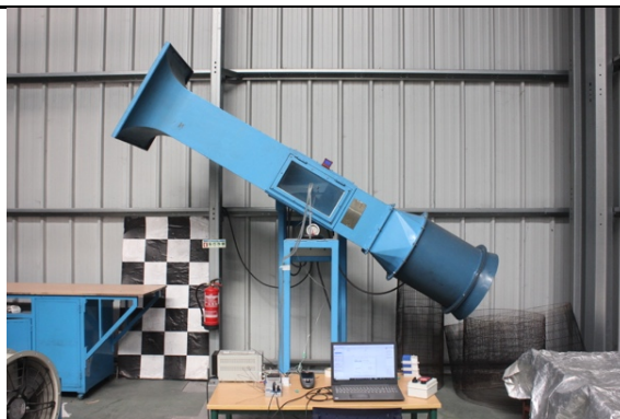
Figure 19: a) Experimental setup scheme (top view) of the S-type Pitot tube in the TCO. b) View the TCO of the Forest Fire Laboratory of the University of Coimbra with three different pitch angles: b1) \alpha_{TCO} = +30^\circ . b2) \alpha_{TCO} = 0^\circ and b3) \alpha_{TCO} = -30^\circ .
