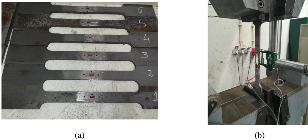
Figure 3.3 – Tensile coupon instrumentation and test set up.
