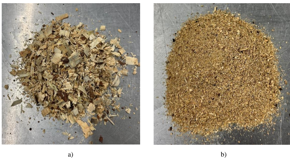
Figure 4.2: Photographic record of the wood aggregates: (a) wood chips (WC); (b) sawdust (SD).
