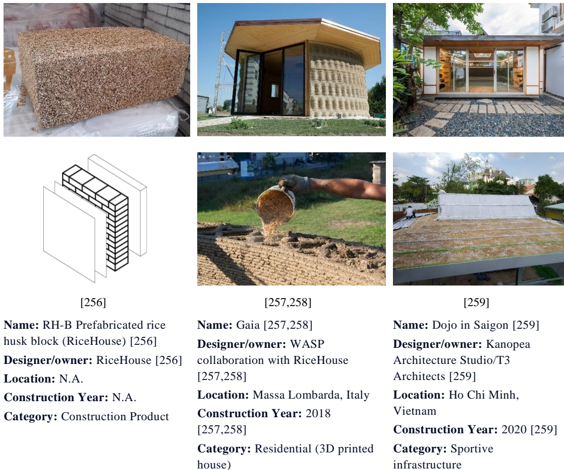
Figure 2.12: Examples of concrete products/projects using rice husk as alternative aggregate.
