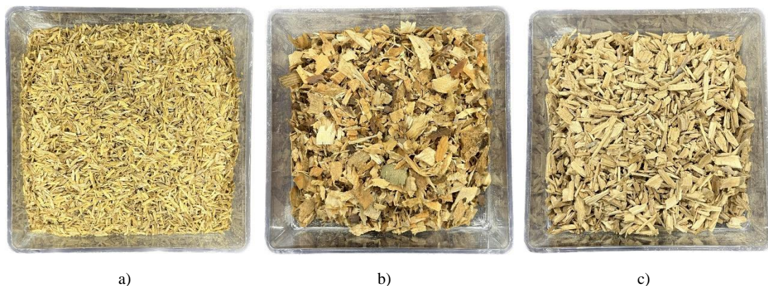
Figure 2.3: Samples of agricultural waste with potential as alternative materials for natural aggregates: a) Rice husk; b) Wood; c) Hemp.
