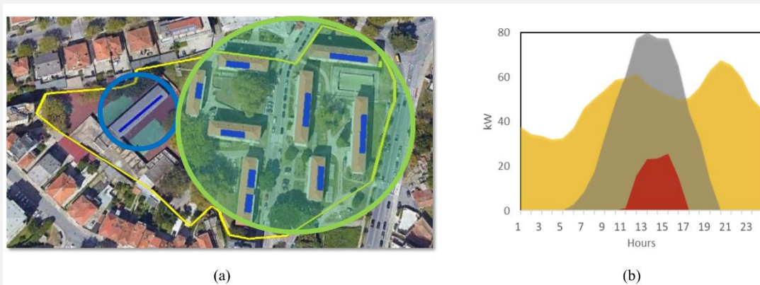
Fig. 15 (a) Surrounding area of the Agra do Amial community, including the school (blue circle) and housing (green circle) and (b) Expected community functioning in a typical summer day, Yellow: demand; grey: generation; red: stored surplus.
