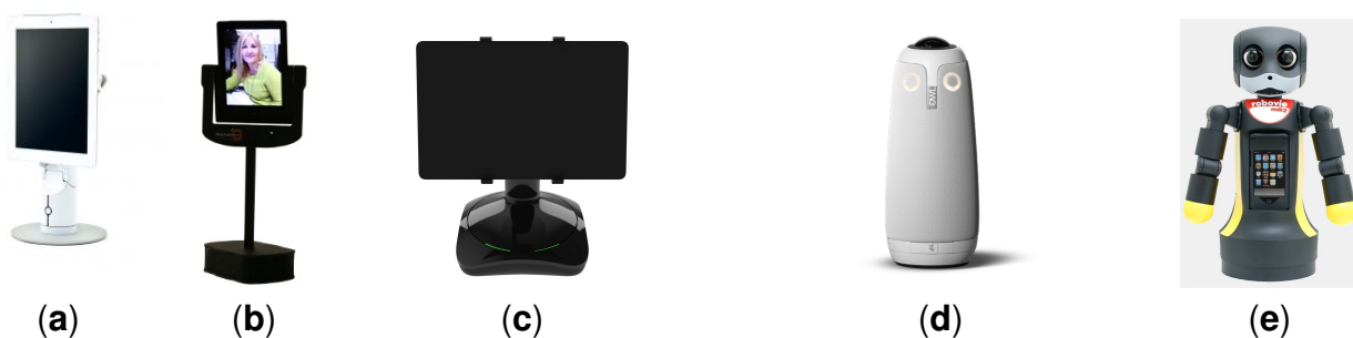
Figure 6.4: Unmovable robotic telepresence (RP) systems: (a) Kubi, (b) TableTop TeleMe, (c) SelfieBot, (d) Meeting Owl Pro, and (e) Robovie mR2.
