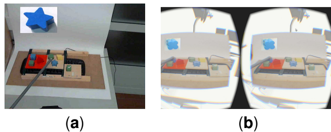
Figure 3.3: Task 1 setup used to compare performances. The user using a hand stick presses a sequence of key blocks defined by the computer at random. Interface view shows the next block to touch at the upper left corner of the display, after each correct touch. (a) Traditional interface vs. (b) immersive interface.
