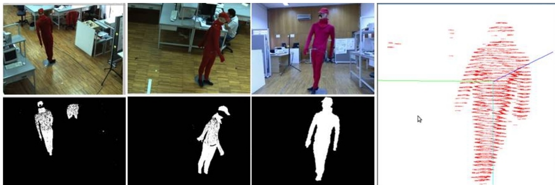
Figure 5.52: Result of 3D reconstruction when a mobile sensor is augmented to the network (corresponding to Fig. 5.51 ); In order to have more details of the scene, a mobile sensor is navigated close to the manikin and its view is integrated as a new node in the network. The left two columns are the images corresponding to the two fixed cameras and the third column from left is the image corresponding to the mobile camera. The results of the 3D reconstruction by using two fixed IS-camera couples and a new augmented couple is demonstrated in the right column.
