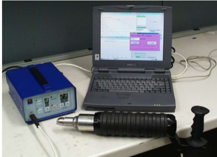
Figure 2.15 – Ultrasonic Impact Technology (Esonix®UIT) equipment [55].
