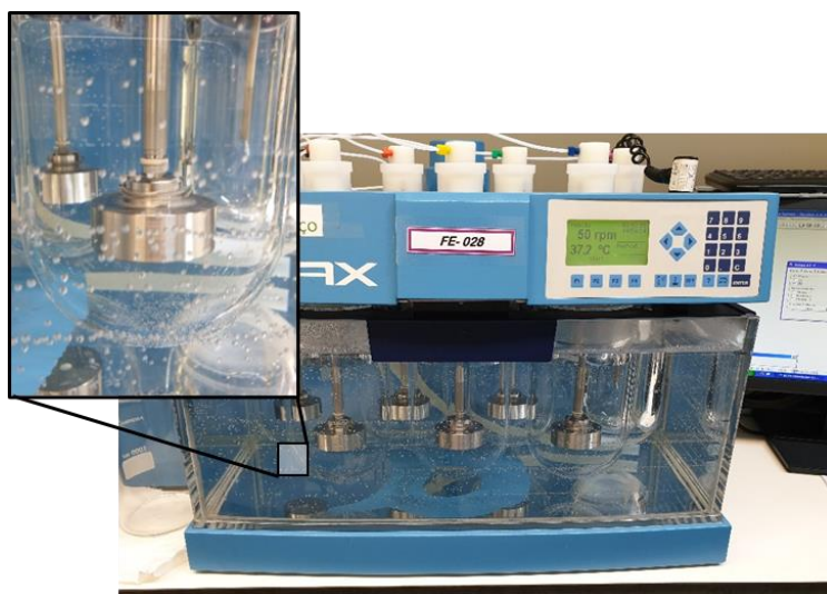
Figure 3.19 SOTAX dissolution rate tester, USP 2 model. Zoom image shows tablet assembled with the shaft and immersed into the 0.01 M HCl solution at time zero.
