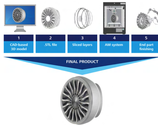
Figure 1.2: General process flow in AM [23].
