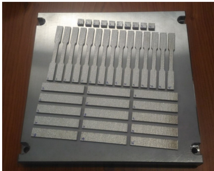
Figure 1. Positions of the specimens on the SLM bed.
