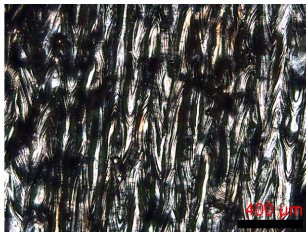
Figure 6.4: Optical micrograph of the 316L stainless steel surface (50x).
