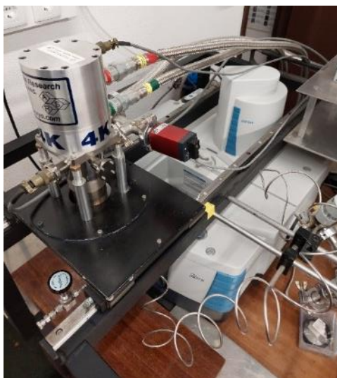
Figure 3 – Thermo Scientific Nicolet iS50 FTIR spectrometer equipped with an MCT/A detector and a KBr beam splitter, mounted together with the ARS Cryogenics closed-cycle helium refrigeration system cryostat used in Section 3.1.
