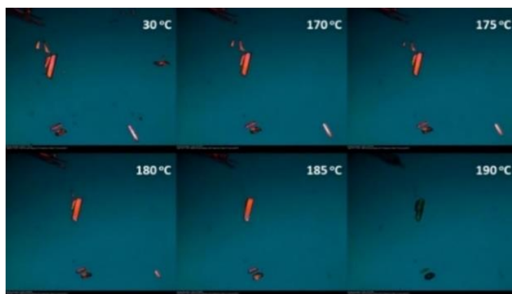
Figure 8 – PLTM images obtained from the heating of the red ROY-CAM polymorph – recrystallized from acetone solution (heating rate: 10\text{ }^{\circ}\text{C min}^{-1} ). These pictures were extracted from the PLTM video1 submitted as Supporting Information.
