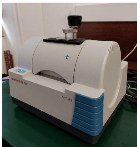
Figure 4 – Thermo Scientific Nicolet iS5 FTIR system, equipped with an iD7 ATR accessory.
