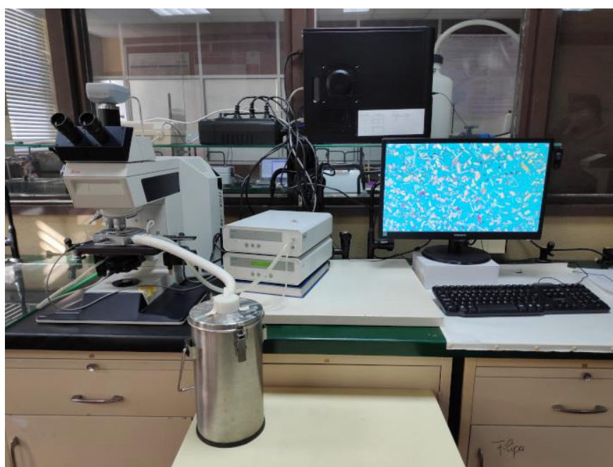
Figure 2 – Linkam DSC-600 hot stage and Leica DMRB microscope with a Sony CCD-IRIS/RGB video camera.
