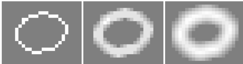
Figure 3.18: Example of “submanifold” dilation. Left: Original curve. Middle: Result of applying a regular 3 \times 3 convolution. Right: Result of applying the same convolution again (Taken from [61]).
