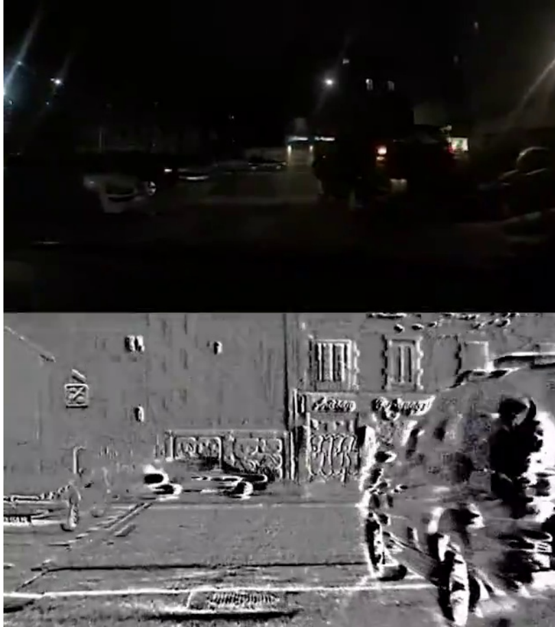
Figure 3.2: Output comparison between frame-based cameras and Neuromorphic vision sensors in terms of low light conditions.
