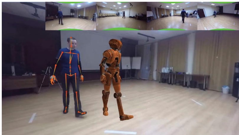
Figure 3.19: Example of how depth information is captured without markers in motion capture [38].
