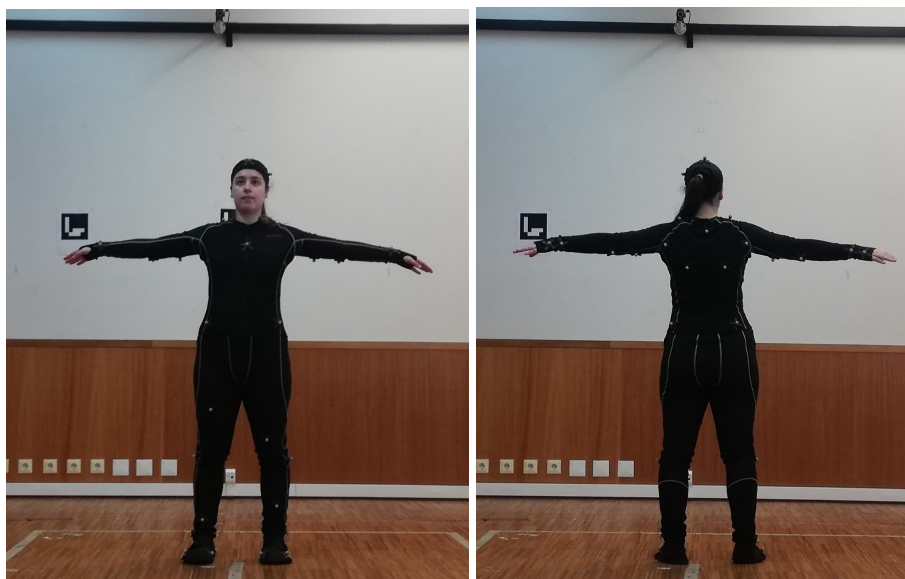
Figure 4.8: Performer equipped with the suit and the 37 markers. Left: front view. Right: back view.
