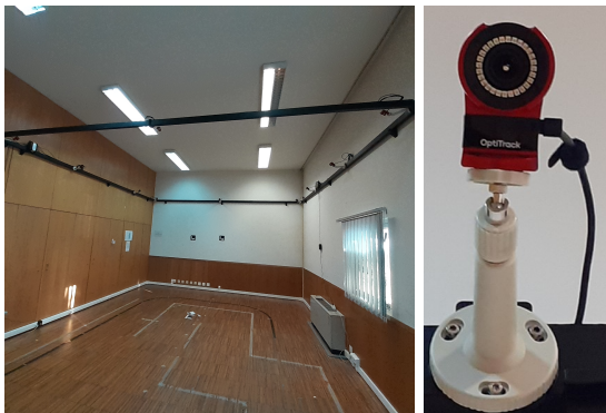
Fig. 4. Left: Motion Capture Room; Right: One of the cameras with its illumination ring visible.
