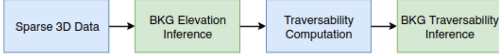
Figure 3.4: Pipeline of Bayesian inference process. Sparse 3D data results in an incomplete elevation map completed with inferred cells that are part of the calculation of the traversability map in place of useless void data.
