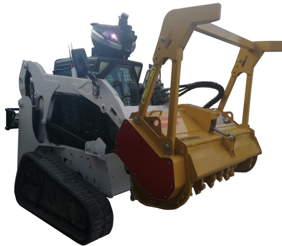
Figure 4.5: Ranger Trials - The Ranger is a tracked vehicle equipped with a mulcher for forest cleanup and sensors for autonomous navigation. At the top of the platform, the LIDAR sensor is aligned with the top of the end effector.
