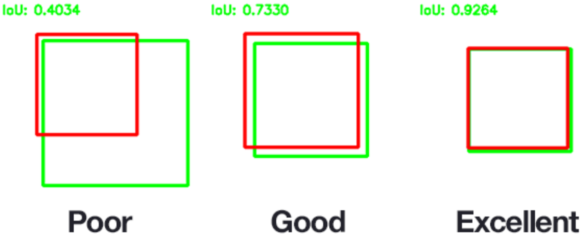
Figure B.2: Intersection over Union - poor, good and excellent score[89]
