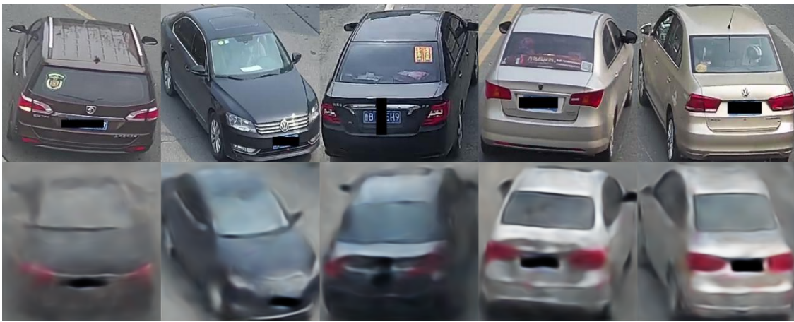
Figure 5.5: Images in their original input form are displayed in the top row, while the second row showcases the output reconstructions produced by the VAE model trained on a limited dataset of 30,000 images.
