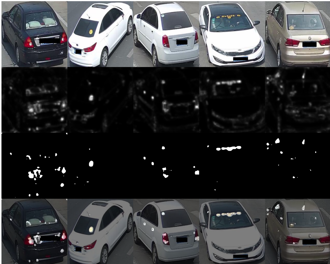
Figure 4.21: In the initial row, the input images are showcased. In the following row, the raw Resnet18 feature map differences are presented. The subsequent row illustrates the final segmentation mask generated with a threshold of 0.3. Finally, the last row exhibits these masks overlaid on the original images, for better visualization.
