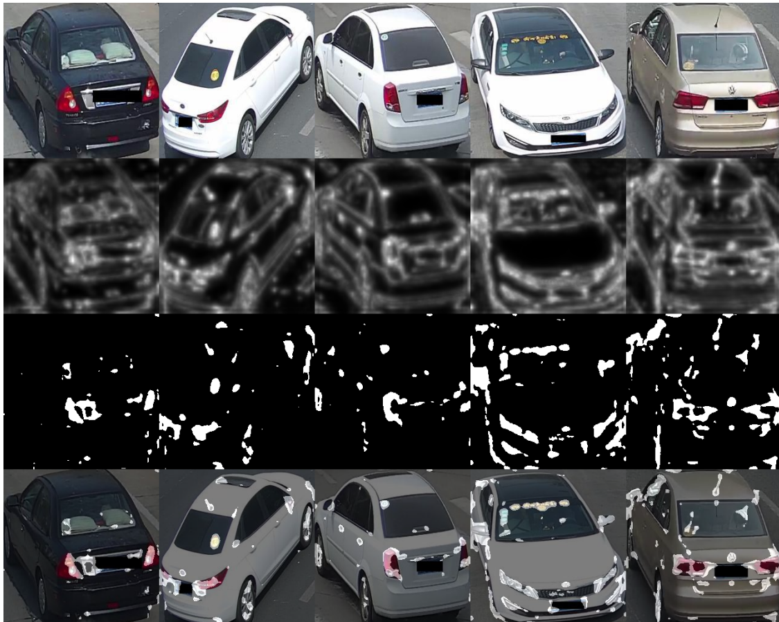
Figure 4.20: The top row highlights the input images, the second row reveals the raw VGG-19 feature map disparities, the subsequent row demonstrates the final segmentation masks created using a threshold of 0.5, and the last row presents these masks superimposed on the original images for improved visualization.
