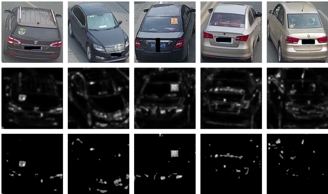
Figure 5.16: Outcomes obtained through the segmentation technique using multi-level Resnet18 feature maps. The top row contains the original images, the second row displays the raw outputs of the technique, and the final row exhibits the thresholded masks with a threshold set at 0.3.
