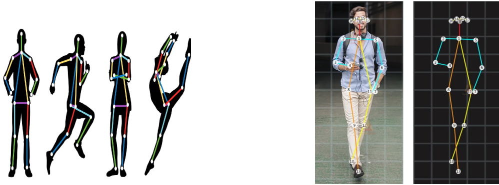
(a) Keypoint capture in a human silhouette [27]. (b) Skeleton keypoint representation of human in a RGB image [28].
