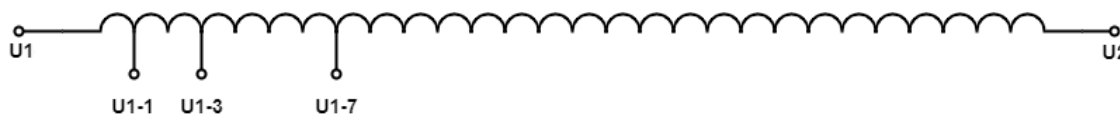
Figure 5.1: Schematic of the stator winding connections that enables the short-circuit between turns.
