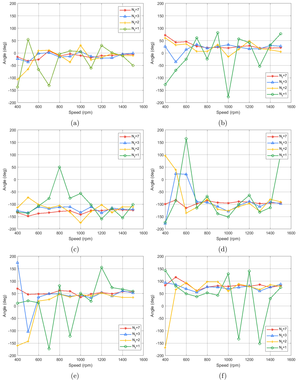
Figure 5.7: Phase variation of e_{\alpha\beta}^- in varying speed conditions: (a) Motor (A1); (b) Generator (A1); (c) Motor (B1); (d) Generator (B1); (e) Motor (A2); (f) Generator (A2).
