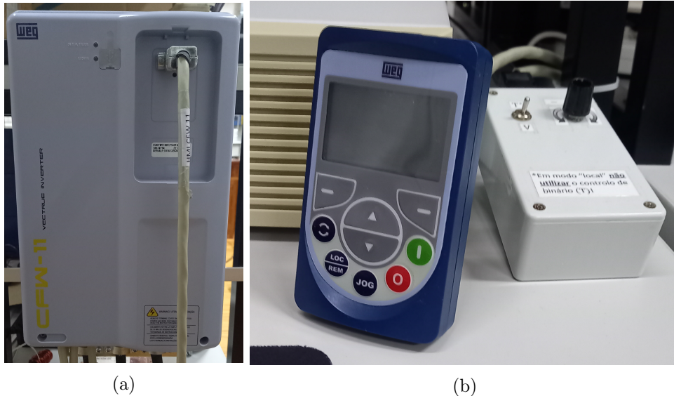
Figure B.2: CFW11 variable speed drive that supplies the IM (a) and remote speed controllers to control the rotational speed of the 6-PMSM (b).
