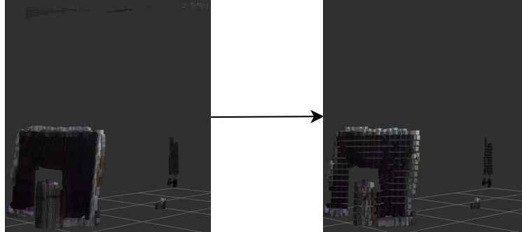
Figure 3.8: Voxelization comparison: left image shows the RoI filtered cloud from 3.6, right image shows the voxelized point cloud. Figure 3.10 illustrates the next step of the pipeline.
