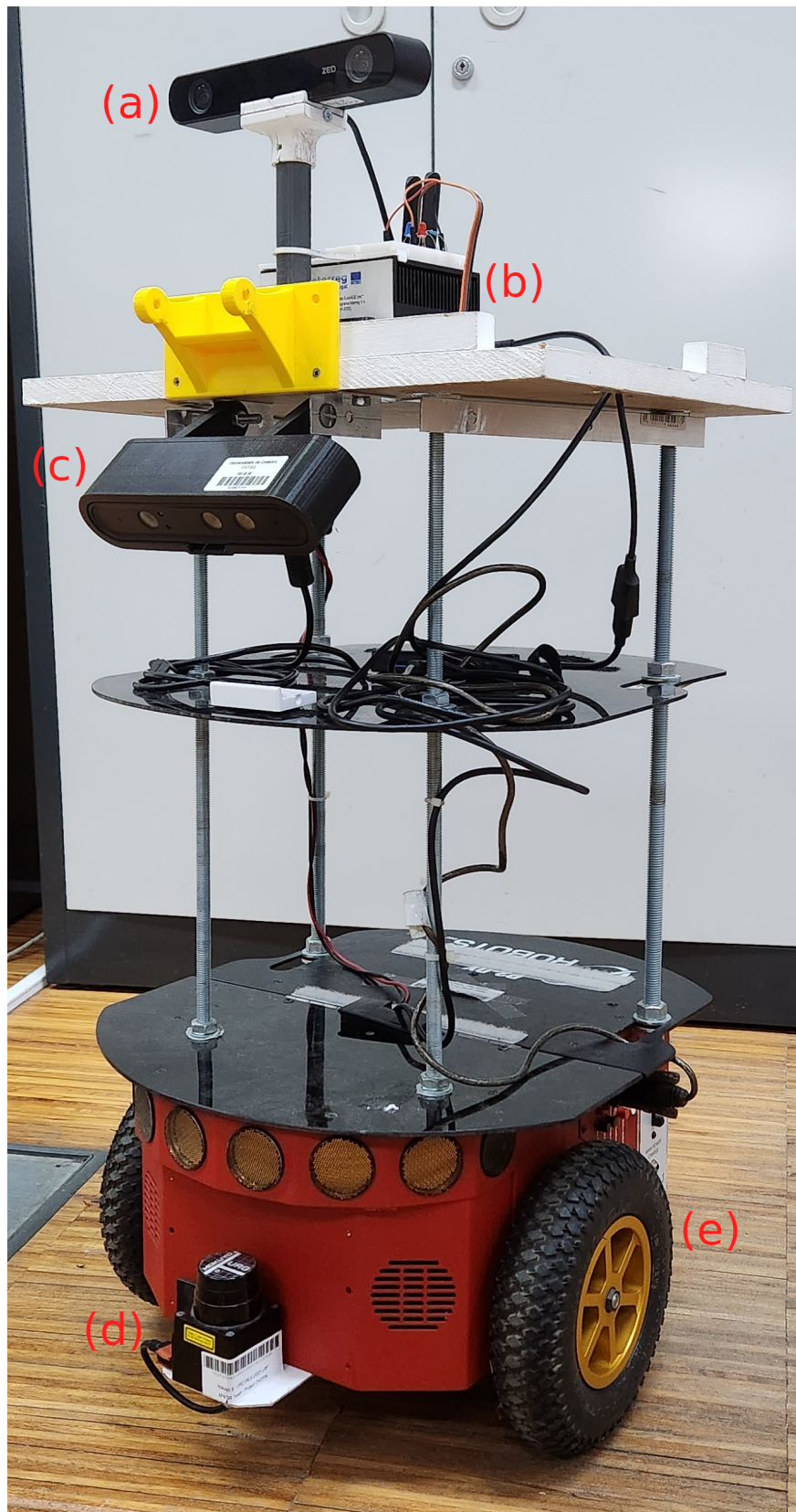
Figure C.6.32: (a) ZED2 Stereo Camera, (b) Jetson AGX Xavier, (c) RGB-D Orbbec Astra, (d) Hokuyo URG-04LX laser range finder, (e) P3-DX Platform.
