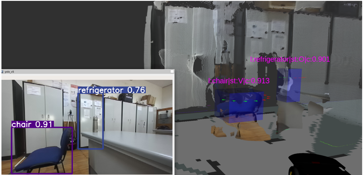
Figure 5.9: SMAP estimation problems. The image displays the map’s problems when observing objects from only one static perspective. The chair is floating due to limited Point Cloud information and the “ refrigerator ” is placed in the wrong position in space (see Section 5.3, page 50). Figures 5.2 and 5.3 explain the indicators present in the figure.
