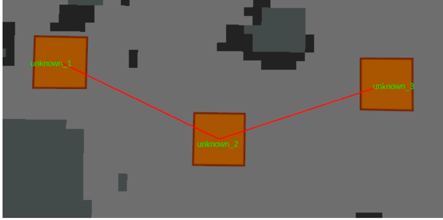
Figure 5.3: SMAP place indicator. The orange squares represent the position of the main vertices of the topological map, the green text is the place classification of this vertice, and the red line shows the connections between vertices (the edges ).
