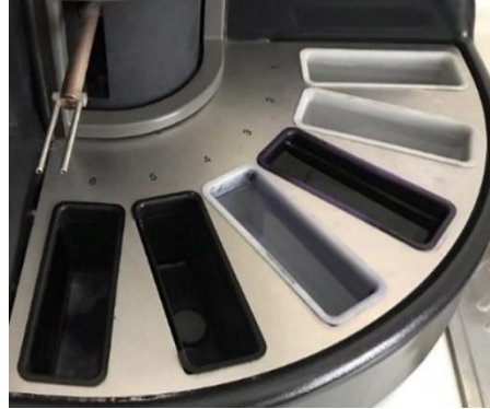
Figure 10: Representation of the 2nd step of G-Banding. Caption: 1- Trypsin solution; 2- Sorensen; 3- Leishman stain; 4- Gurr; 5-H 2 O; 6- hot air.
