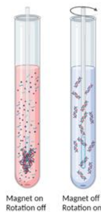
Figure 12: Magnet beads function representation of the Prepito technique. Done In Biorender (chemagen Technologie GmbH, 2023a).
