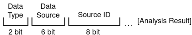
Figure A.3: This is the Id data format for the Analysis data.
