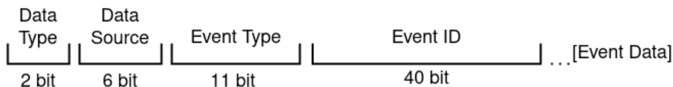
Figure A.1: This is the ID data format for the Physics Event data.
