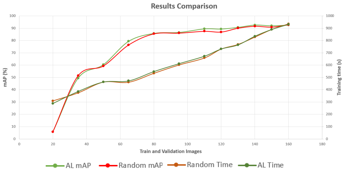
Figure 5.1: Comparison Chart: mAP achieved with incremental number of images used in training and validation, selected via Active Learning (AL) vs Random Selection. Training time comparison included.
