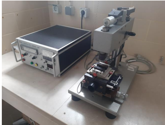
Figure 8) Scratch test device used in this work
