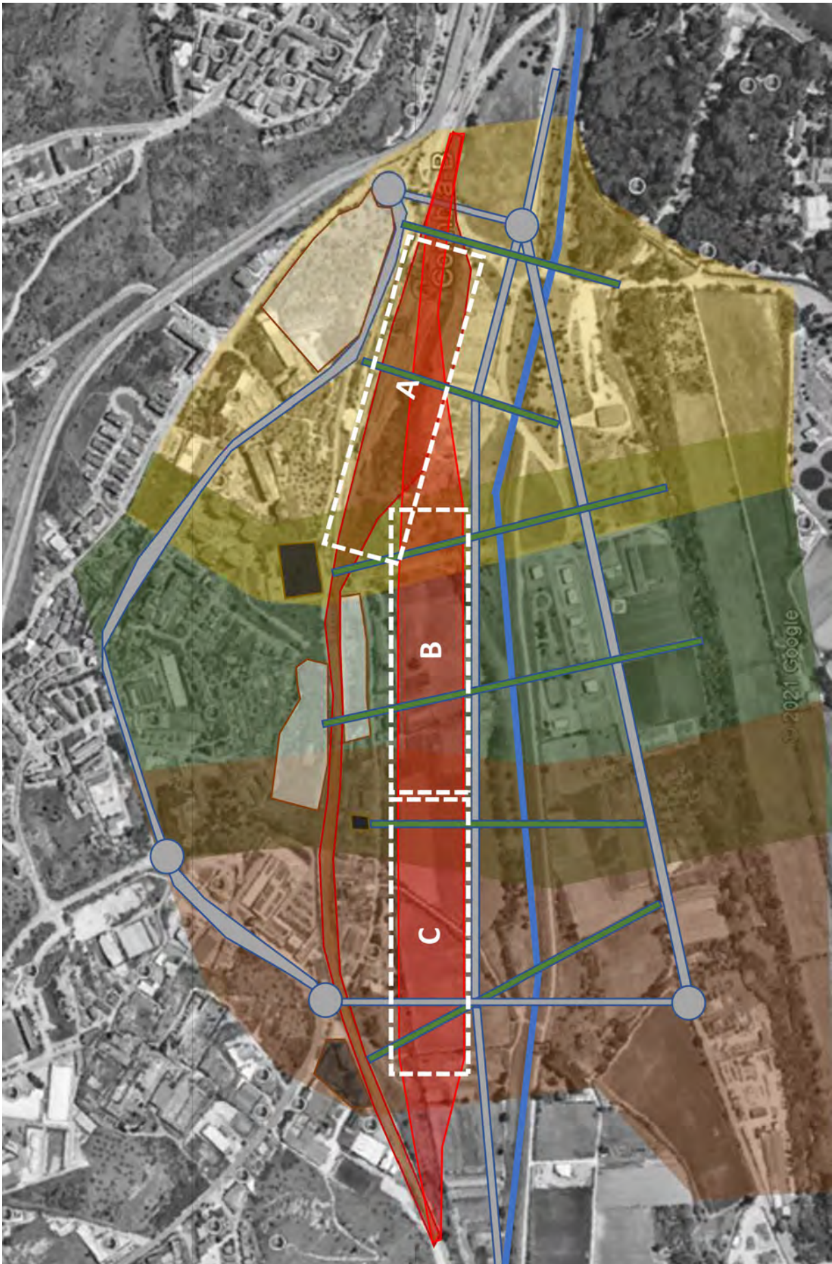
Figure 1: Diagram for groups A, B and C - Different placements for the railway station.
