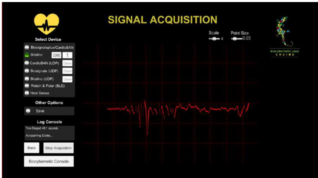
Figure 5.5 - BLE receiving the Bitalino signal via Bluetooth.
