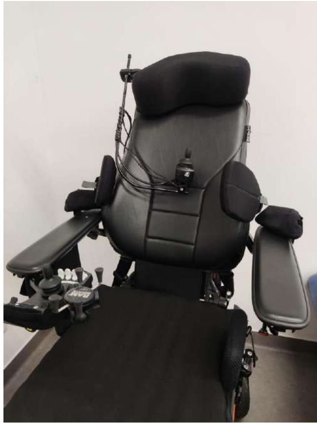
Figure 2.10 - Electric wheelchair with a chin and hand manipulation control. Captured in a visit to APELA.
