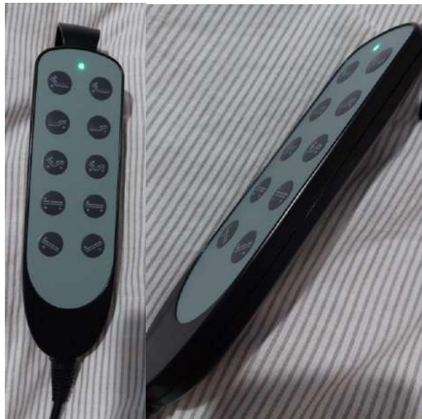
Figure 4.3 - Controller used and described by the interviewee to change her bed’s position. Captured by the interviewee.
