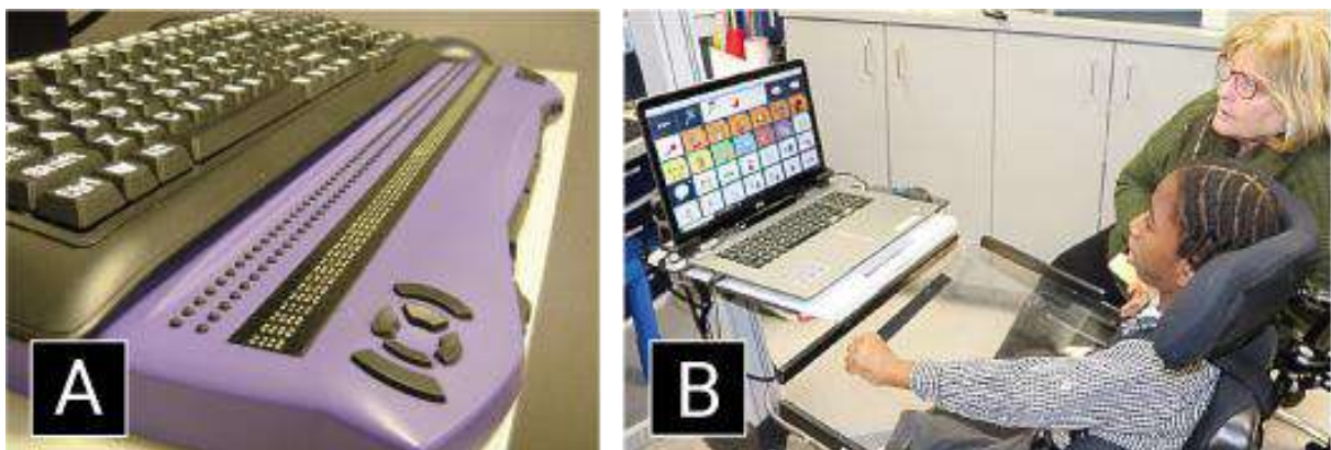
Figure 2.9 - Examples of hard technologies of assistive technologies. (A) keyboard with key input for typing and braille output for reading, (B) conjugation of two assistive technologies: electric wheelchair; laptop with portable Tobii eye gaze system and Communicator 5 software.
