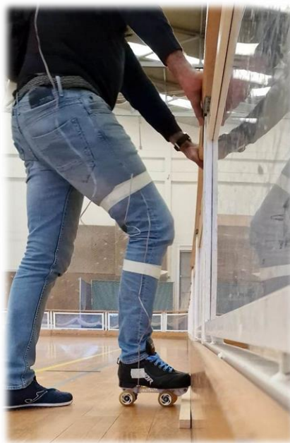
Figure 5.5. Final testing setup on the athlete; Roller skate platform without the braking device.
