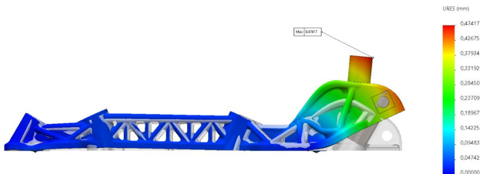
Figure 4.22. FIB corrected static numerical study: Resultant displacement plot; ABS.
