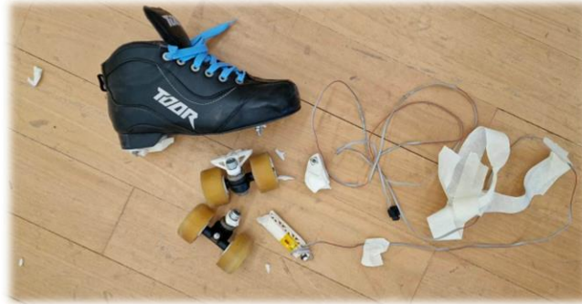
Figure 5.6. Roller skate after failure and the removal of the boot by the athlete.
