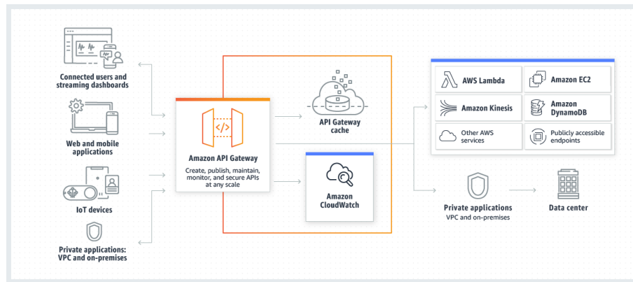
Figure 4.3: Amazon API Gateway architecture.
