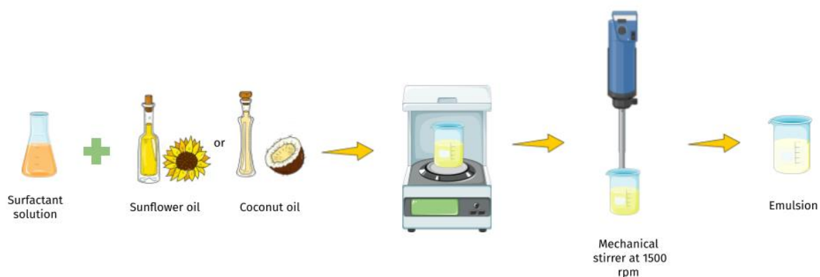
Figure 17: Process of emulsion production using mechanical stirring.
