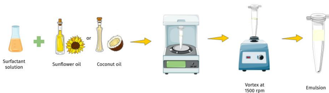
Figure 15: Procedure of emulsion preparation using vortex.
