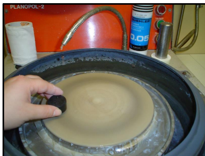
Figure 10 - Manual polishing of the samples.
