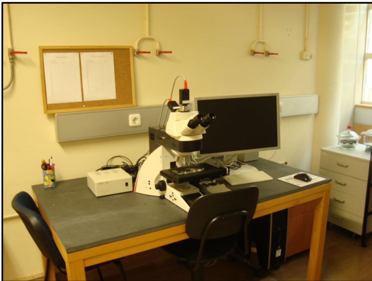
Figure 12 - Leica DM4000 microscope, equipped with the software "Discus-Fossil" from Technisches Büro Hilgers.
