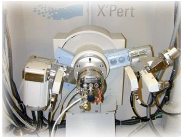
Fig. 4.3: Internal arrangement of a PHILIPS X'Pert PRO X-ray diffractometer
