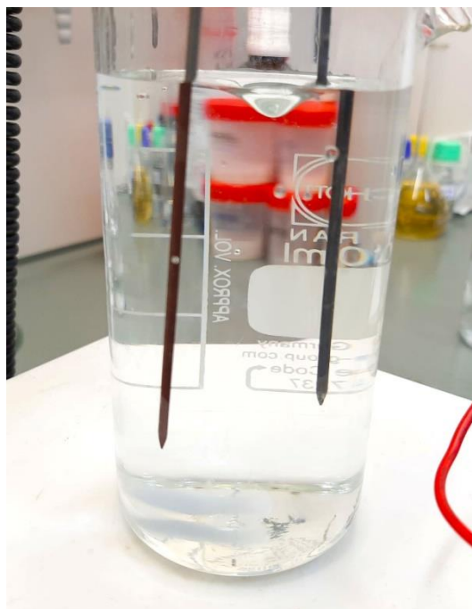
Figure 40 - Copper deposition on the cathode.
