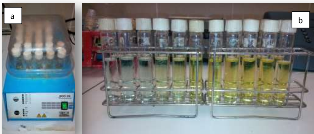
Figure 12 - Illustration of samples in COD determination. (a) Samples in the thermo-reactor. (b) Samples before absorbance reading.
