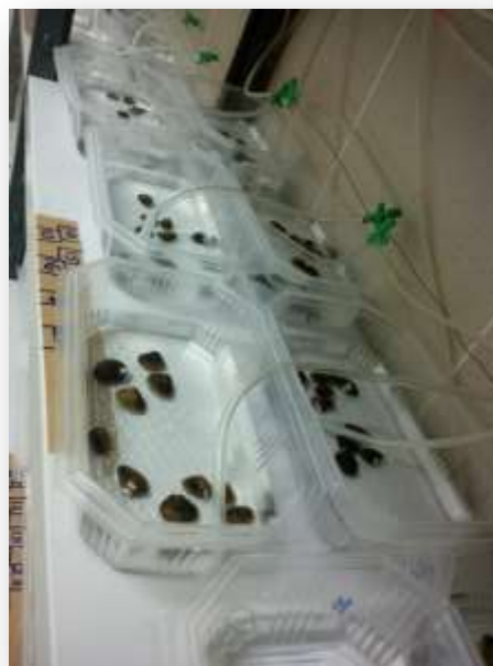
Figure 13 - Set-up for the mortality tests with Asian clams.
