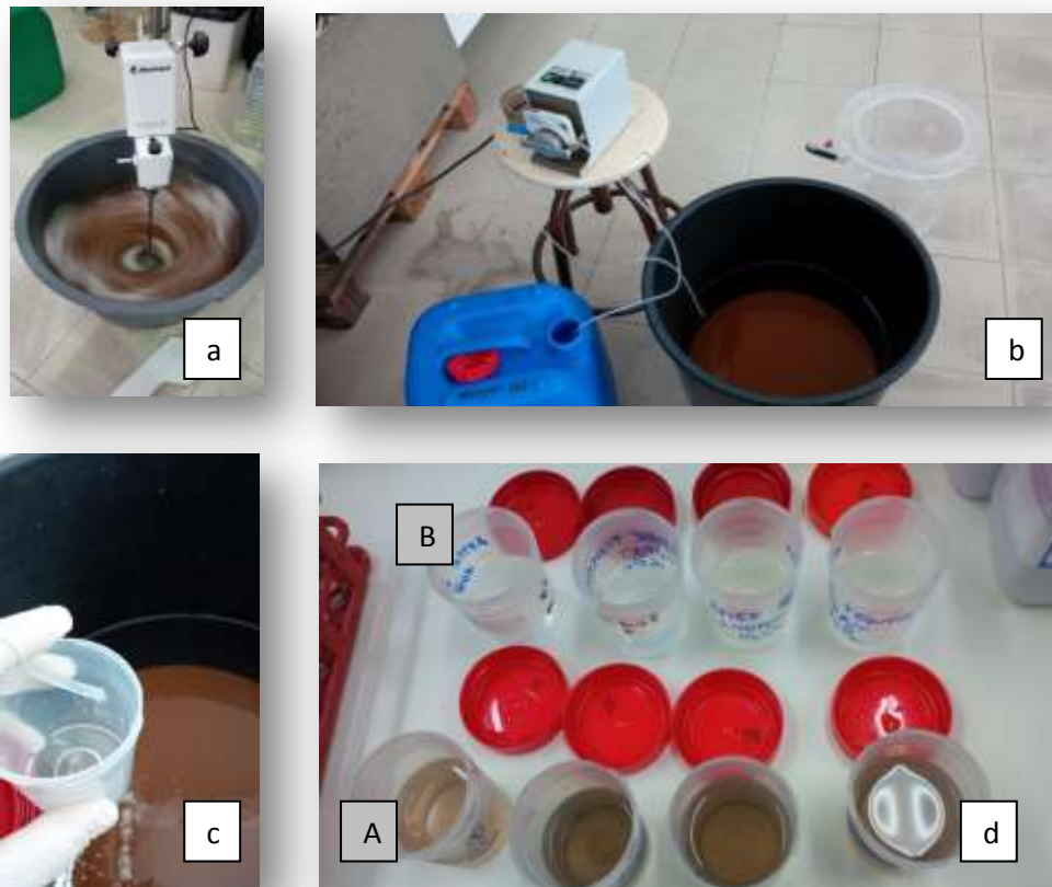
Figure 5 - Treating the winery effluent by Fenton's reaction. (a) Fenton reaction involving 16 hours of continuous stirring. (b) Sedimentation after stopping Fenton's reaction. (c) Fenton-treated effluent separation from Fe-rich sediment. (d) Effluent (A) before and (B) after Fenton's reaction (original and Fenton-treated samples, respectively).
