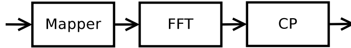
Figure 2.2: Basic waveform of OFDM transmitter that can implement the digital back-end of the radio architecture shown in Fig. 2.1).
