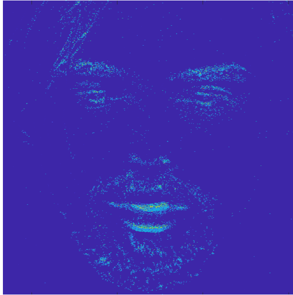
Figure 8: Example of an Accumulation of Exponential Time Surface Frame: This is a AETS frame of a user face integrated during 40ms .
