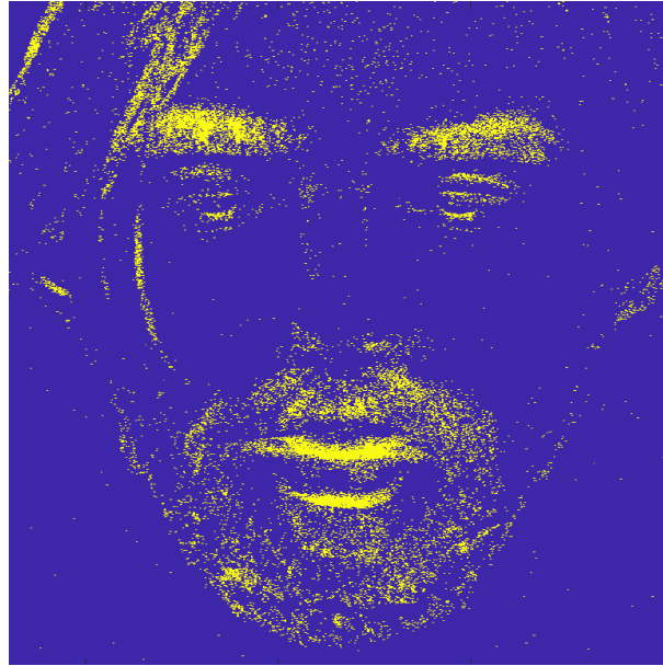
Figure 3: Example of a Binary Event Frame: This is a Binary Event frame of a user face integrated during 40ms . The yellow frame pixels have the maximum intensity, whereas the dark blue colored pixels have the lowest intensity.
