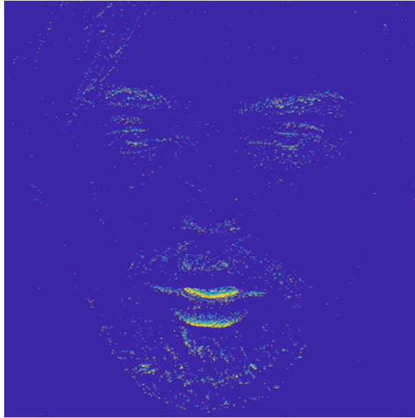
Figure 6: Example of a Surface of Active Events Frame: This is a SAE frame of a user face integrated during 40ms . It is noticeable that this representation, while low on noise, has the dynamic features of the face highly emphasized.
