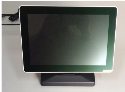
Figure 4.1: The TT electroadhesion haptic technology developed by Tanvas and the four available objects used in the tests.
