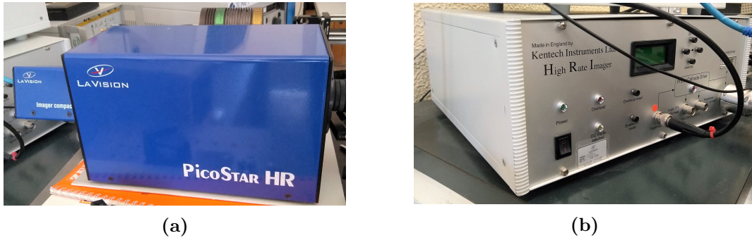
Figure 3.6: The HRI (figure 3.6a) and its controller module (figure 3.6b) from LaVision.
