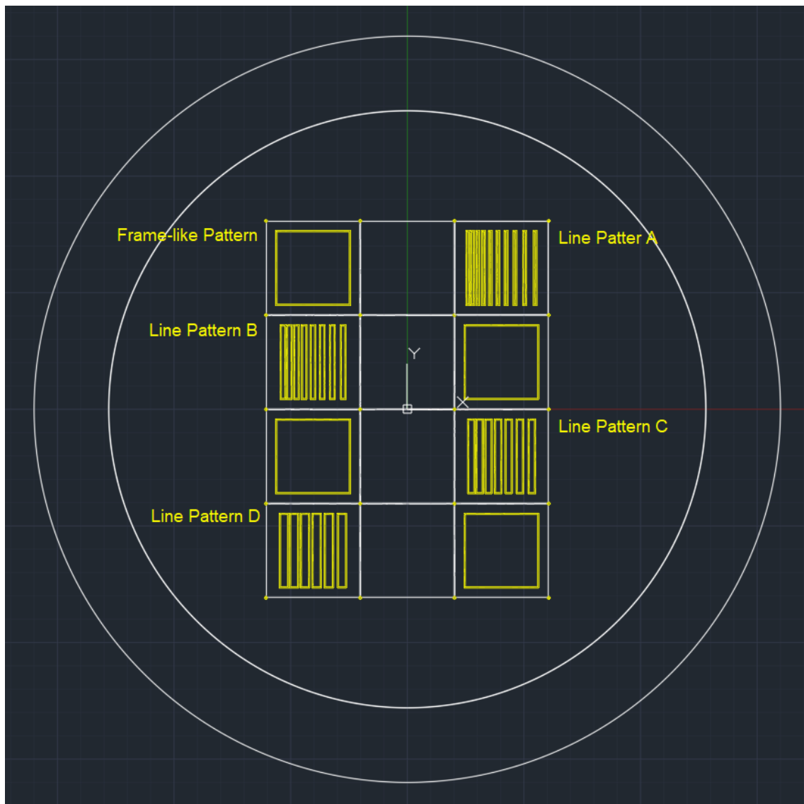
Figure A.1: Print screen of the AutoCAD design of the developed shadow mask.
