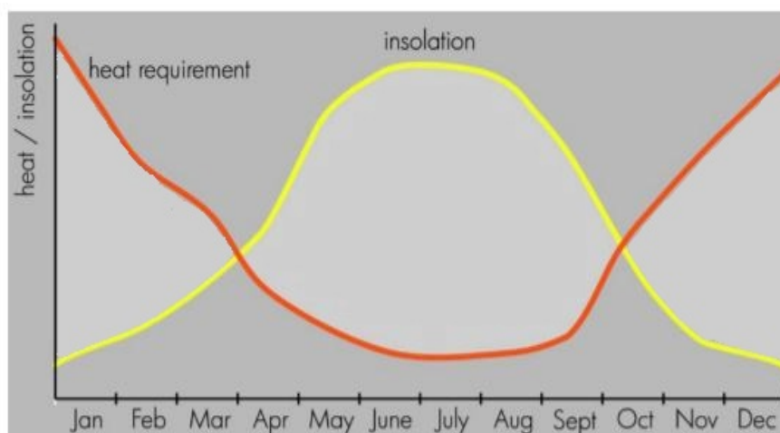
Figure 1.3: Solar heat supply in the summer (middle) and heating demand during the winter (left and right) (adapted from Solites (2016)).
