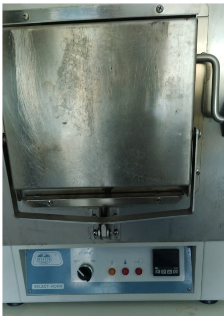
Figura 4.5: Mufla P-SELECTA SELECT-HORN .
