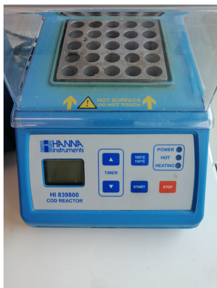
(a) Termo reator HI 839800, HANNA Instruments.
