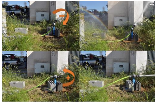
Figure 3.11 - Pump on vs pump off; On top: 60-degrees assembly; on bottom: 0-degrees
