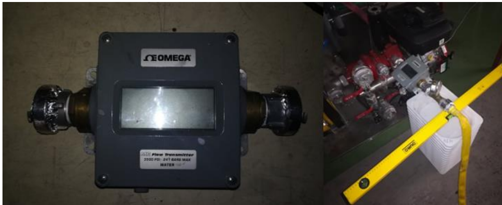
Figure 3.28 - Flowmeter and its assembly
