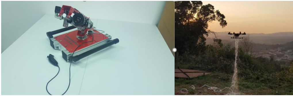
Figure 1.4 - Two referred firefighting technologies; 1) on the left the portable water monitor; 2) on the right, the drone
