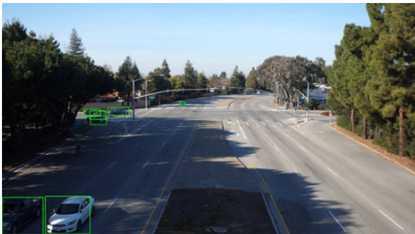
Figure 4.4: Vehicle detection with three different F-RCNN proposed in [1]
