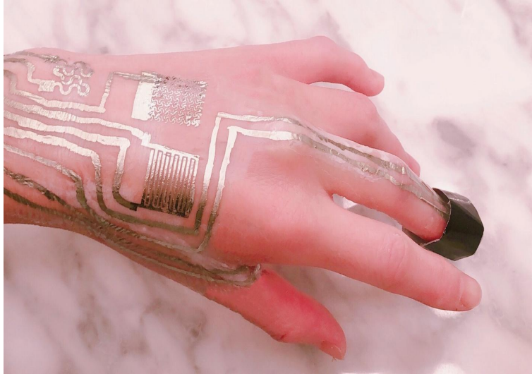
Figure 1.3: Circuit directly sintered on human skin at room temperature [9]
