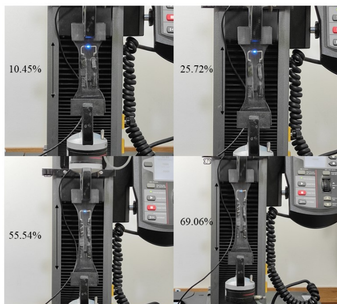
Figure 4.19: Stretching a battery and analyzing the brightness of the LED for each strain value.
