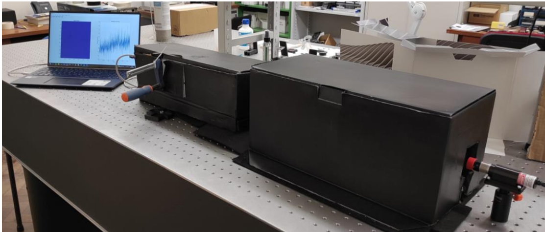
Figure 4.3 – Prototype assembled in the optical table, including the host computer, the acquisition branch-box, the transmission and excitation branches-box, and finally, the laser.
