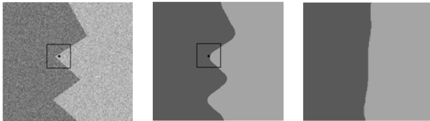
Figure 2.16: Illustration of the smoothing effect. (left) Synthetic image containing two regions with different Gaussian noises. (middle) Segmentation result using the method proposed in [3]. (right) Segmentation result with a very large integration scale
