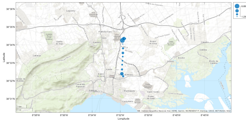
Figure 3.15: Location and R_{Gi} values for each pylon i in LPM.SB1 line.
