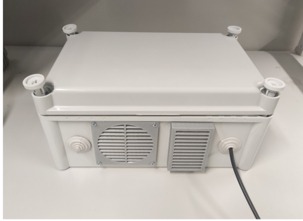
Figure 4.11: Outside view of the power supply casing.
