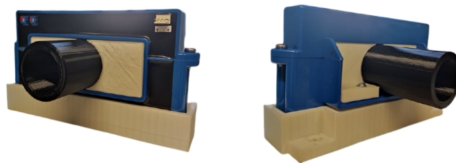
Figure 4.8: 3D printed pieces to embrace the neutral cable. Black cylinder imitates neutral cable.
