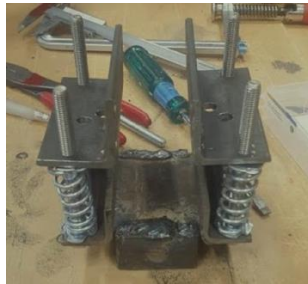
Figure 2.9. Complete suspension unit (Dzezhyts, 2020).
