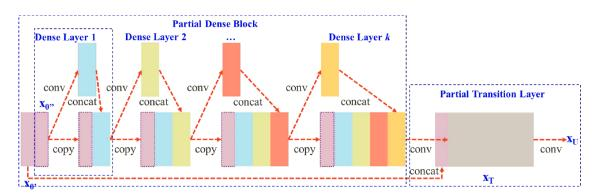
Figure 3.3: Partial CSPDarknet53 Architecture. [68]
