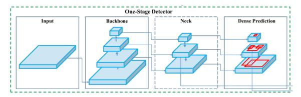
Figure 3.2: YoloV4 Architecture. From: [20]
