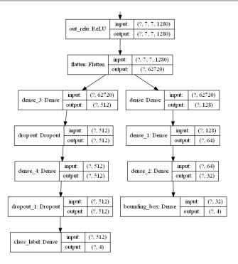
Figure 4.1: Naive model arquitecture after the last output from MobileNetV2.
