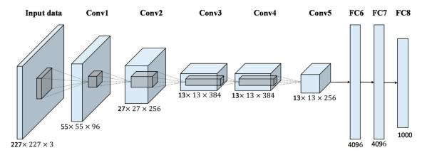
Figure 2.6: AlexNet: Convolutional Neural Network. From: [40]
