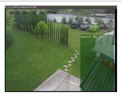
Figure 5.8: SSD-MobileNetV2 detection on Jetson.
