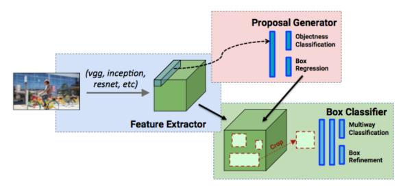
Figure 3.6: Meta-architecture for Two Stage Detectors. From: [34].
