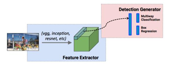
Figure 3.1: Meta-architecture for One Stage Detectors. From: [34].
